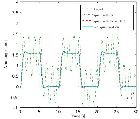
**Fig. 4.** Arm angles without quantization and with quantization by our error feedback quantizer (dashed line) as well as by the static quantizer (long dashed short dashed line).
