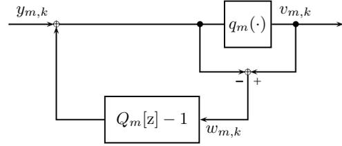
Fig. 2. Quantizer with an error feedback filter
