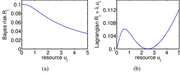
**Fig. 1.** (a) The Bayes risk  $R_i(u_i; \boldsymbol{\xi}_i)$  is a non-convex function of  $u_i$ . (b) The Lagrangian in (9) can have more than one minimizer.
