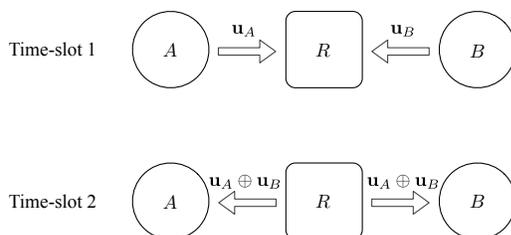
**Fig. 1.** A three-node TWRC applying the PNC concept.
