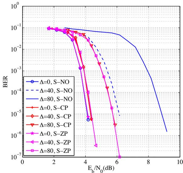
**Fig. 5.** BER performance of the system using no compensation, CP and ZP at different arrival delays.
