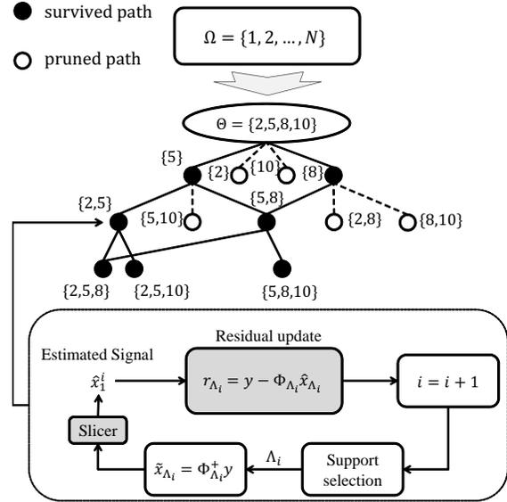
Fig. 1. Illustration of proposed SDMP algorithm.
