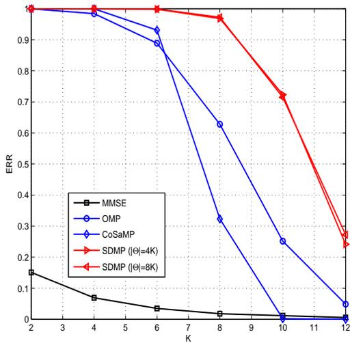
**Fig. 2.** ERR performance of sparse detection at SNR = 25 (dB).
