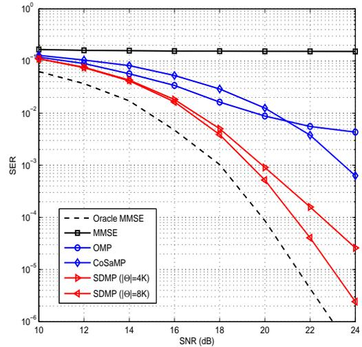
**Fig. 3.** SER performance of sparse detection when  $K = 5$ .
