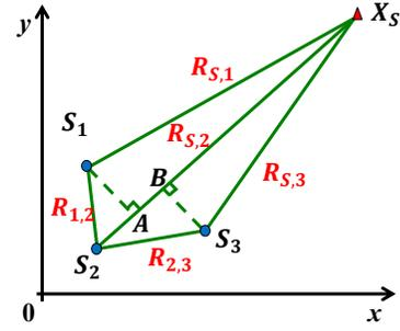
**Fig. 2.** Sensor locations and impact location. The circles  $\mathbf{S}_1, \mathbf{S}_2$  and  $\mathbf{S}_3$  denote sensor locations and the triangle  $\mathbf{X}_S$  denotes the impact location.  $\mathbf{S}_1\mathbf{A} \perp \mathbf{X}_S\mathbf{S}_2$  and  $\mathbf{S}_3\mathbf{B} \perp \mathbf{X}_S\mathbf{S}_2$ .
