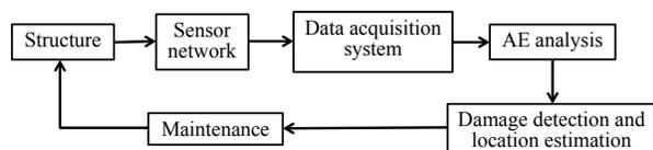
**Fig. 1.** A generic block diagram of an impact location estimation system.
