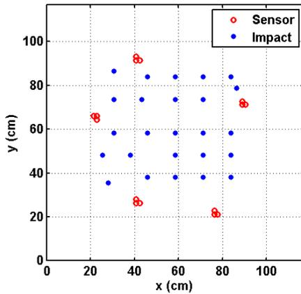
**Fig. 3.** Sensor distribution on the quasi-isotropic carbon/epoxy panel.
