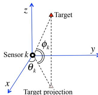
**Fig. 1:** AOA sensor measurements in 3D space.
