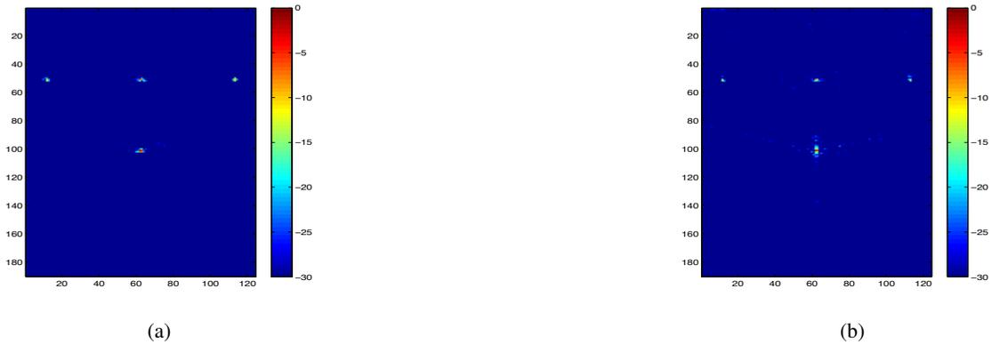
**Fig. 2.** Field II simulated program with four point scatterers and 128 elements uniform linear array of transducers. (a) image reconstructed with the Capon beamformer and (b) image reconstructed with the CS recovery based on the regularized- $l_1$  method followed by applying the Capon beamformer to the recovered signals. Both figures used the same 30-dB display dynamic range.
