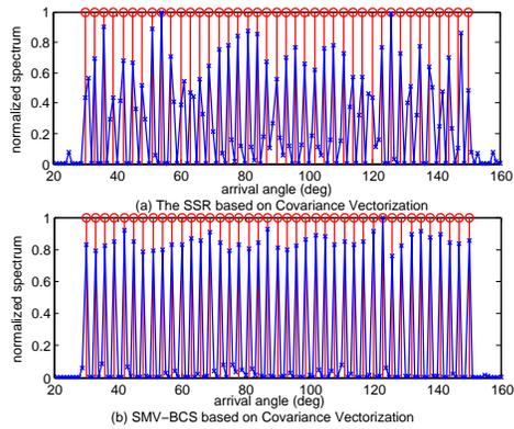
Fig. 2: Sensing spectra of two DOA estimation algorithms for partially augmentable arrays.
