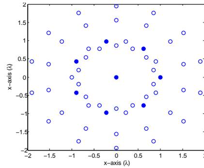
Fig. 3: The 8-antenna circular array and its difference coarray.
