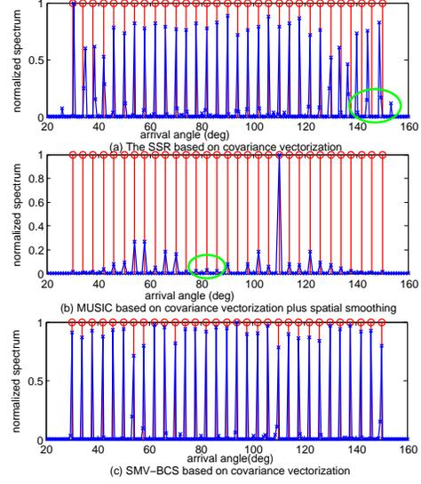
Fig. 1: Sensing spectra of three DOA estimation algorithms for fully augmentable arrays.
