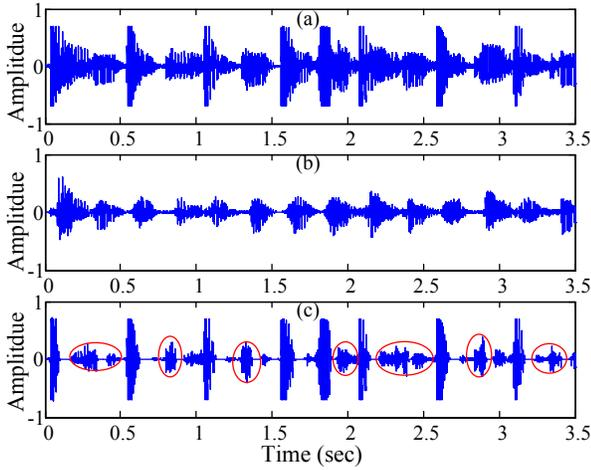
Figure 4. Steady-state and transient separation using median-filter based method. a) The input signal. b) The separated steady-state signal. c) The separated transient signal. (Note: the circles indicate steady-state components contained in the separated transient signal.
