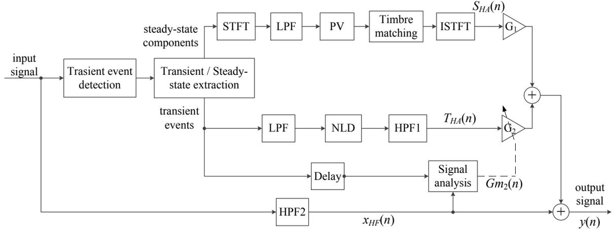
Figure 3. General framework of the proposed VBS with gain control. (STFT and ISTFT: short-time Fourier transform and inverse short-time Fourier transform; LPF and HPF: low-pass and high-pass filters; PV and NLD: the phase vocoder and the nonlinear device;  $x_{HF}(n)$ : high-frequency components of the input signal;  $S_{HA}(n)$  and  $T_{HA}(n)$ : synthesized harmonics of steady-state and transient components;  $Gm_2(n)$ : maximum gain for harmonics).
