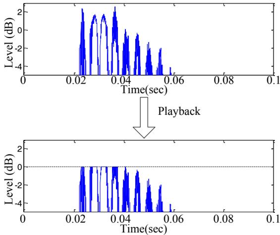
Figure 2. Clipping distortion in the playback due to the arithmetic overflow of the signal.
