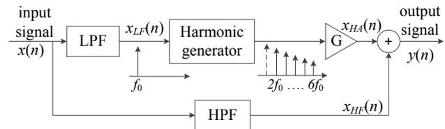
Figure 1. General framework of the VBS. (LPF and HPF: low-pass and high-pass filters; G: gain for harmonics;  $x(n)$  and  $y(n)$ : input and out signal, where  $n$  represents the sample index;  $x_{LF}(n)$  and  $x_{HF}(n)$ : low-frequency and high-frequency components of the input signal;  $f_0$ : the fundamental frequency;  $x_{HA}(n)$ : synthesized harmonics).
