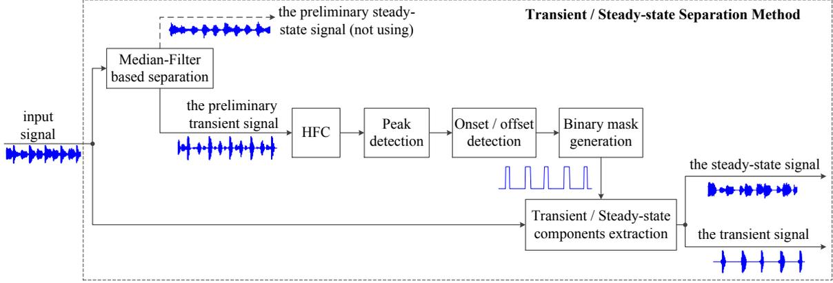
Figure 5. Processing blocks of the proposed steady-state and transient separation method.
