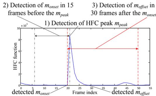
Figure 6. Detection of transient events using the HFC function. ( $m_{peak}$ : the peak frame,  $m_{onset}$ : the onset frame,  $m_{offset}$ : the offset frame;  $- \cdot -$ : detection range for  $m_{onset}$ ,  $- - -$ : detection range for  $m_{offset}$ )
