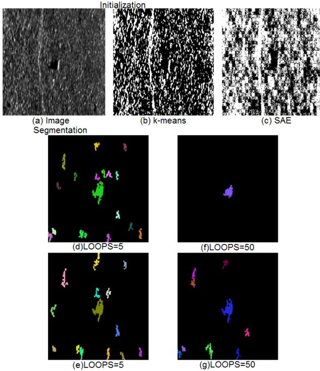
**Fig. 4.** Label field initialization and the MRF segmentation for an image taken by a side-scan sonar.
