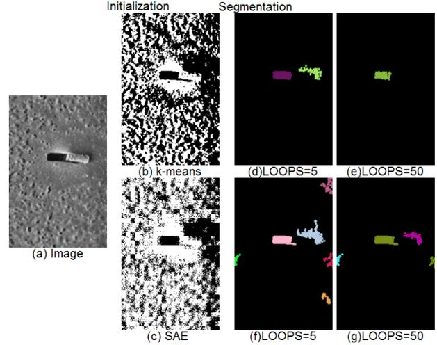
**Fig. 5.** Label field initialization and the MRF segmentation for an image taken by a multi-beam high-resolution sonar.
