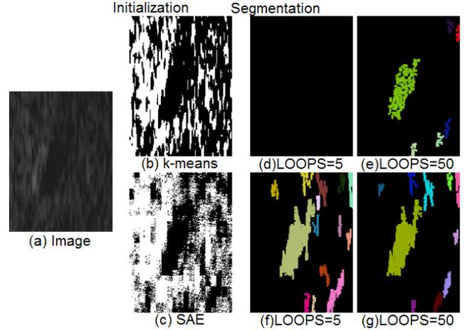
**Fig. 3.** Label field initialization and the MRF segmentation for an image taken by a forward-looking sonar.(a) is the original image, (b) and (c) is the initial label field obtained by *k-means* algorithm and the proposed SAE method respectively. The corresponding image segmentation results are shown in (d) and (f) for 5 loops, (e) and (g) for 50 loops.“*LOOPS*” is the iterations in the ICM method.
