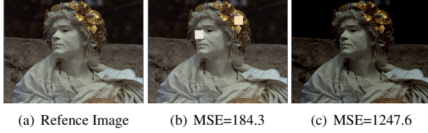
Fig. 2. The images are from the public database TID2008 [15]. (a) is a reference image, (b) is distorted with only two small white blocks, (c) is distorted with entirety intensity shift.
