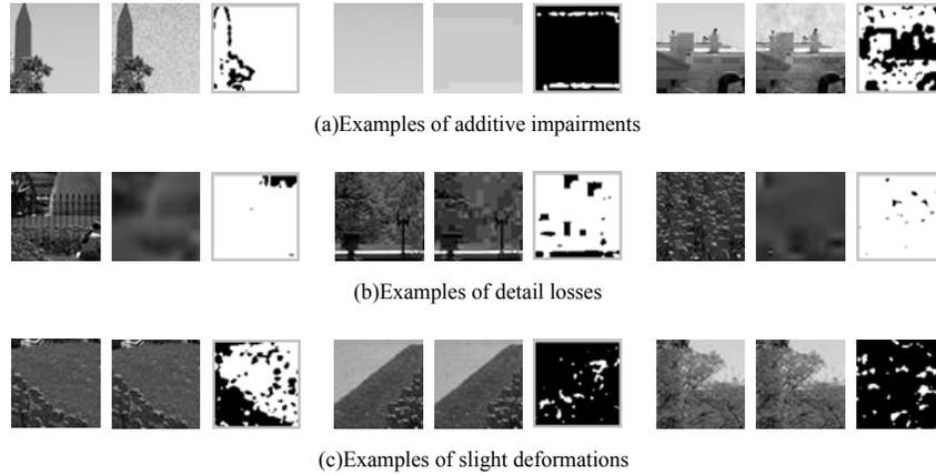
Fig. 1. Examples of the patches used in the experiments and their classifications. Each groups of (a), (b) and (c) has three kind images. The left and middle images are original and distorted images for each. The right images are the map using structure component of SSIM, in which the white parts means the value of the pixel is lower than 0.9.
