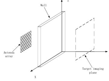
Fig. 1. Typical TWGI using ghost imaging scenario
