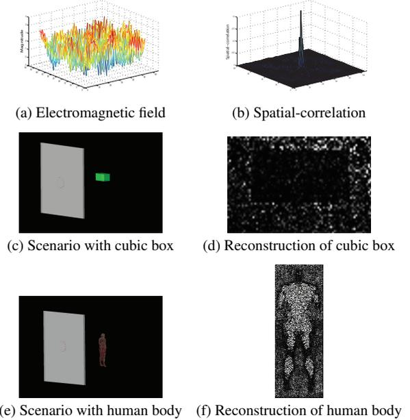
Fig. 4. Detecting signal and EM field at target imaging plane.
