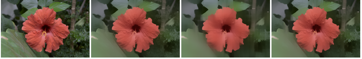
Fig. 2: The bilateral filtering results (“flower”): from left to right, input image, naïve, conventional separable implementation, and proposed separable implementation. The filtering parameters are \sigma_c = 65 , \sigma_s = 16.33 , r = 49 , and \alpha = 0.8 for the proposed. The computational time is 450 ms (naïve), 16 ms (conventional) and 17 ms (proposed).
