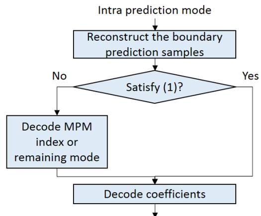
**Fig. 5.** Flowchart of decoding CU for bitstreams encoded using Redundant Bits Removal (RBR).
