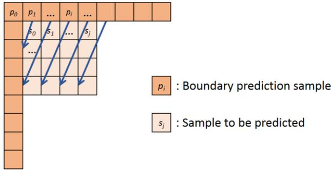
**Fig. 1.** Illustration of intra prediction for an CU in HEVC using boundary samples.
