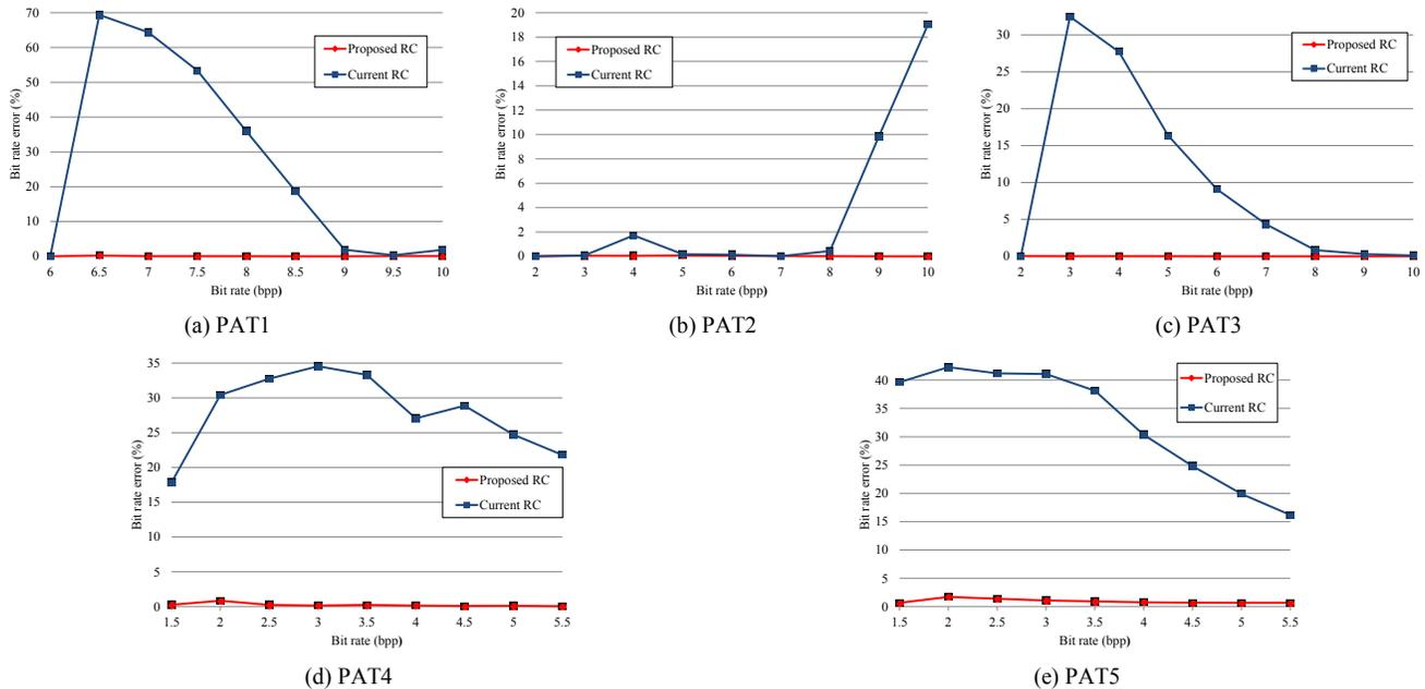
Fig. 2. Bit rate error, in percentage, of the proposed and current RC algorithms for different bit rates and test images. In all cases, the RoI is encoded losslessly. Bit rates shown correspond to overall bit rates (RoI + BG).
