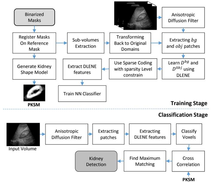
**Fig. 1.** Displaying block diagram of the kidney detection.
