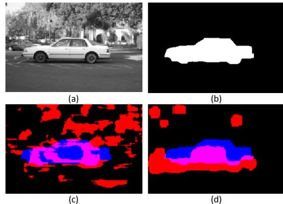
**Fig. 2.** Classifying pixels belonging to a car from the caltech-101 database [19]. (a) original image, (b) binarized mask, (c) D-KSVD, and (d) DLENE-NN.
