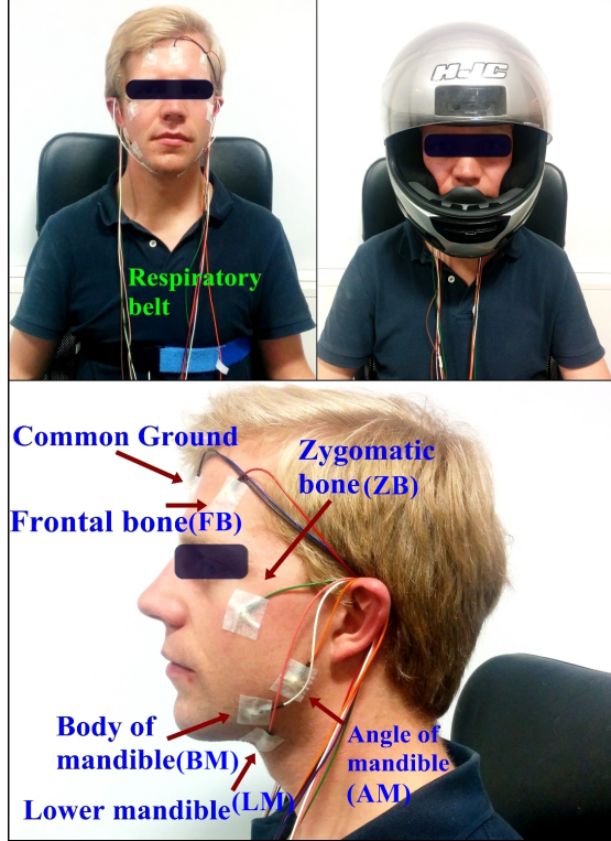
Fig. 1: The standard limb-lead ECG, respiratory signal and face-lead setup (top-left). The subject wearing a racing helmet with the face-lead configuration (above-right). Electrodes were attached to five locations on the face, the zygomatic bone, frontal bone, angle of mandible, body of mandible and lower mandible (lower).
