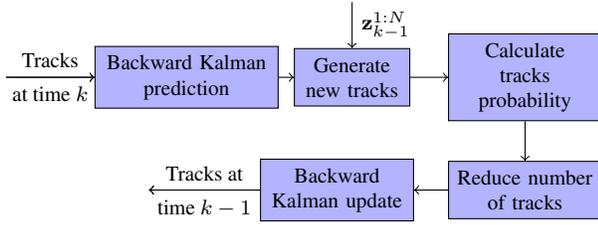
**Fig. 3.** Flowchart of multiple hypothesis Kalman filtering.
