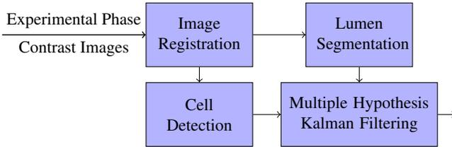
**Fig. 2.** Diagram of the proposed automated multi-cell tracking system.
