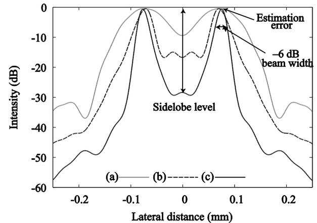
**Fig. 3.** Cross-sectional images at a 50 mm depth using (a) a DAS method, (b) a conventional BS Capon with sub-array size of 32 element and diagonal loading factor of  $-20$  dB, and (c) the BS Capon method with proposed method.
