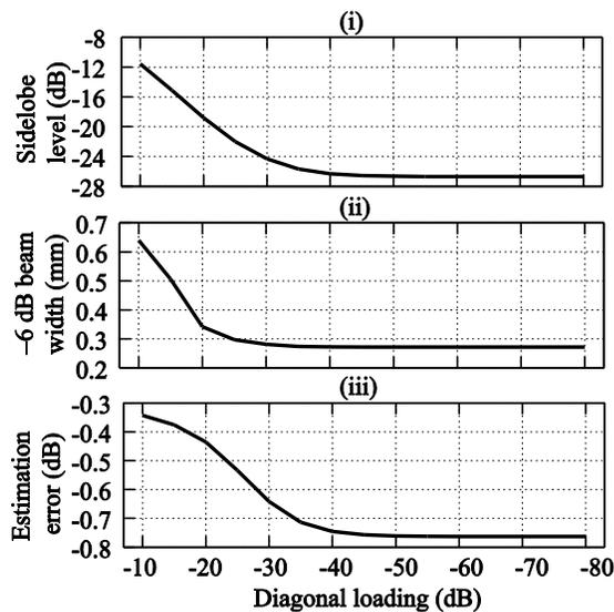
**Fig. 4.** (i) Sidelobe level, (ii)  $-6$  dB beam width, and (iii) estimation error in intensity using proposed method, where the diagonal loading factor was ranges from  $-10$  dB to  $-80$  dB.
