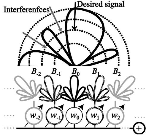
Fig 1. Schematic of a BS Capon beamformer.
