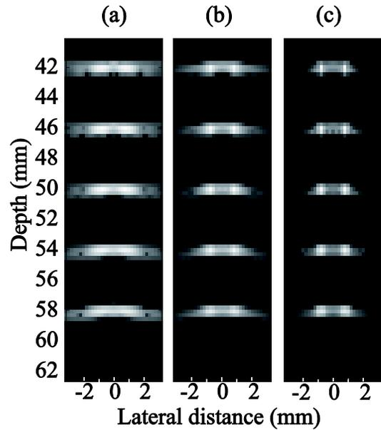
**Fig. 2.** B-mode images of point targets using (a) a DAS method, (b) a conventional BS Capon with the sub-array size of 32 elements and a diagonal loading factor of  $-20$  dB, and (c) a BS Capon method with the proposed technique and diagonal loading factor of  $-40$  dB. The dynamic range is 60 dB. Target depths were 42 mm, 46 mm, 50 mm, 54 mm, and 58 mm.
