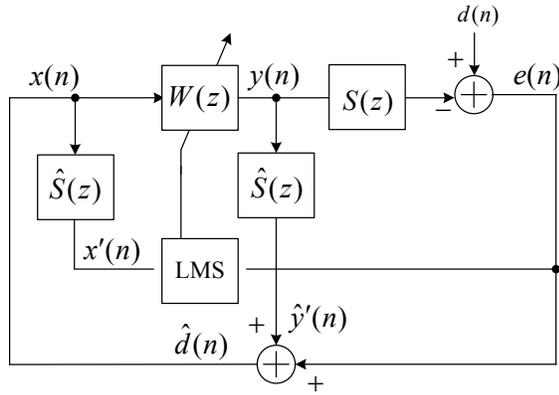
Fig. 1. Block diagram of a typical adaptive feedback ANC system.
