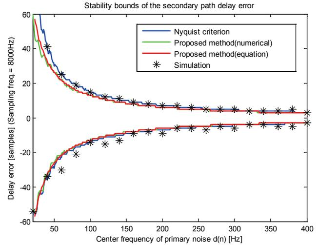
Fig.4. Comparison of stability bounds obtained with different methods. Stability bound obtained by Nyquist criterion(Blue), Numerically obtained bound of condition (4) (green), Bound obtained by equation (12) (red), and Simulation results (stars).
