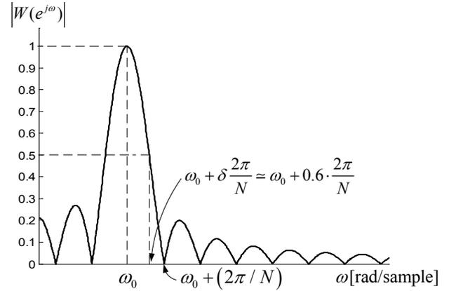
Fig.3. The magnitude response of the optimum ANC filter,  $|W_o(e^{j\omega})|$  for single-tone sinusoidal primary noise.
