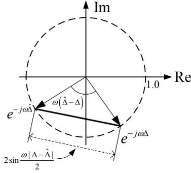
Fig.2. The magnitude of  $e^{-j\omega\Delta} - e^{-j\omega\hat{\Delta}}$  illustrated in the complex plane.
