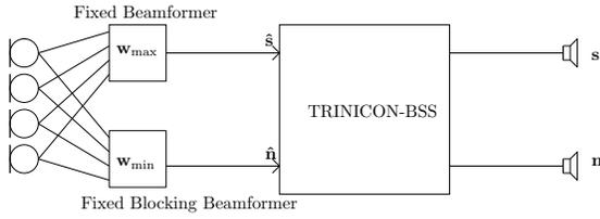
**Fig. 1.** System design. The two imperfect beamformer outputs are fed into the TRINICON-BSS system to exploit the minimum mutual information property of BSS algorithms to compensate for imperfections inherent in realistic scenarios.
