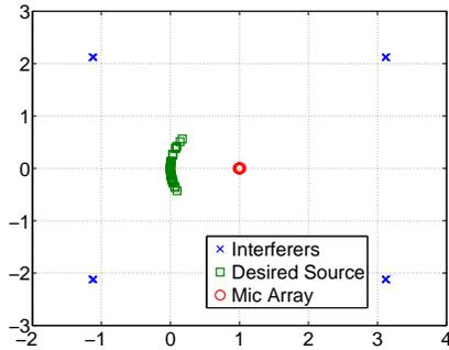
**Fig. 3.** Monte Carlo simulation of source positions (in metres), interferer locations, and microphone layout.
