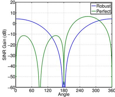
**Fig. 2.** Example of the expected SINR gain for the robust and (typical) perfect blocking beamformers. Plots are shown for a 4-element 2 cm radius circular array at 550Hz.
