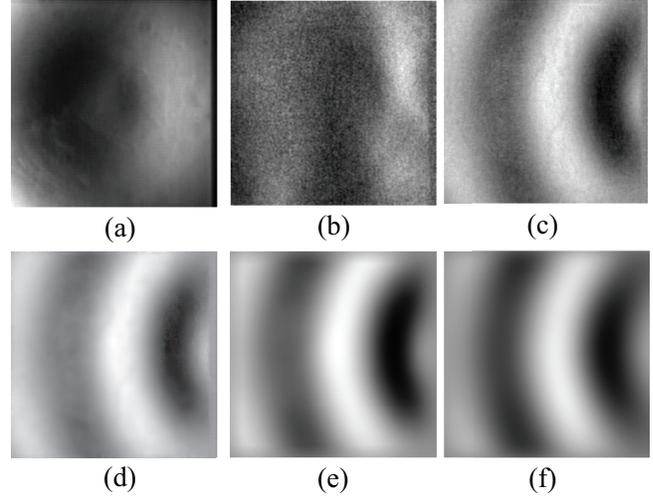
**Fig. 4.** 10 kHz sinusoidal sound field. (a) Measured data, (b) data without DC component, (c) time directional filtering by bandpass filter, (d) spatio-temporal filtering by bandpass and Wiener filter, (e) spatio-temporal filtering by bandpass and Gaussian filter, (f) spatio-temporal filtering by 3D Gabor filter.
