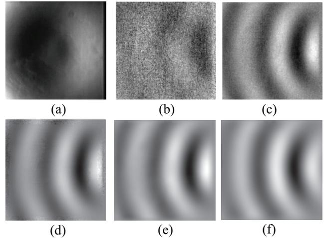
**Fig. 5.** 15 kHz sinusoidal sound field. (a) Measured data, (b) data without DC component, (c) time directional filtering by bandpass filter, (d) spatio-temporal filtering by bandpass and Wiener filter, (e) spatio-temporal filtering by bandpass and Gaussian filter, (f) spatio-temporal filtering by 3D Gabor filter.
