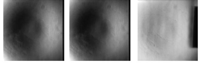
**Fig. 2.** Schlieren images of 10 kHz, 15 kHz and 40 kHz sinusoidal sound fields detected by a high-speed camera.
