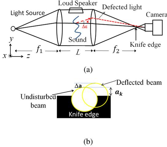
**Fig. 1.** Drawing of Schlieren system and the displacement of the light beam. (a) two-lens Schlieren system with  $f_1 = 100$  cm,  $f_2 = 102$  cm and  $L = 100$ , (b) horizontal displacement of light beam.
