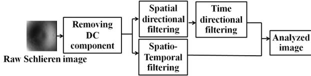
**Fig. 3.** Procedure of visualization of sound field
