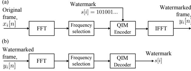
**Fig. 3.** General scheme of the proposed method: (a) process of embedding one bit and (b) process of detecting one bit.
