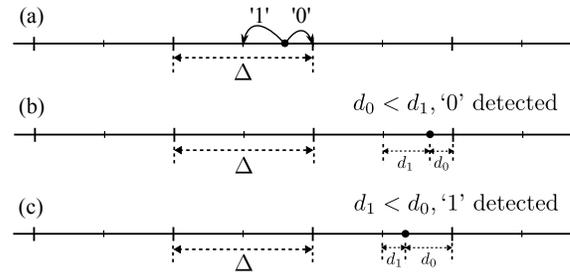
**Fig. 1.** An illustration of QIM-based watermarking technique: (a) embedding, (b) detection of ‘0’, and (c) detection of ‘1’.
