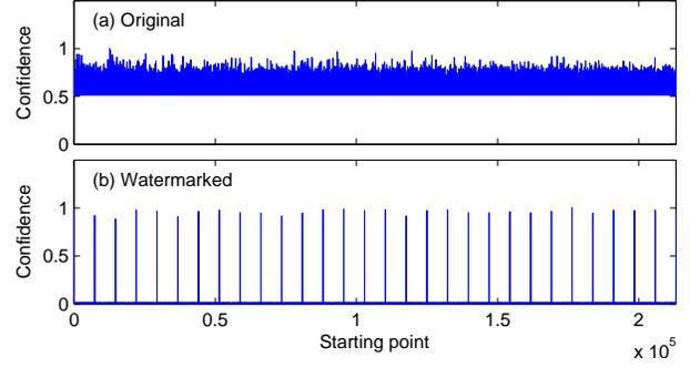
**Fig. 4.** An illustration of frame position detection in the case frame length = 7350 points: (a) original signal and (b) watermarked signal.
