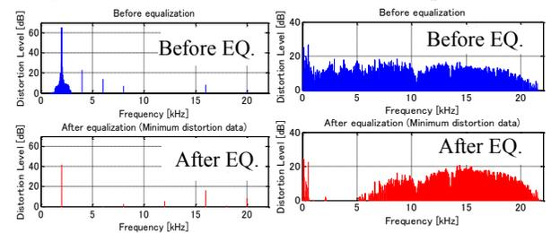
Fig. 9. Amplitude spectrum with/without equalization
