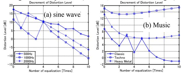
Fig. 8. Distortion level vs. Number of equalizations
