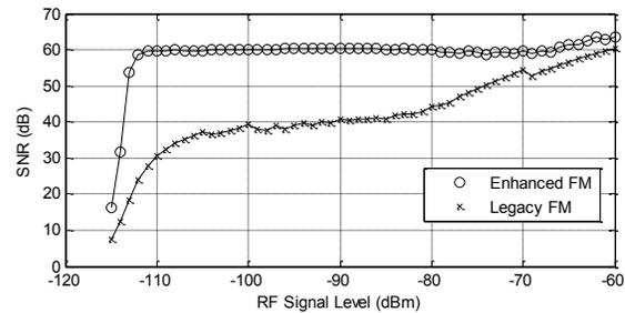
Figure 5 SNR versus RF signal level
