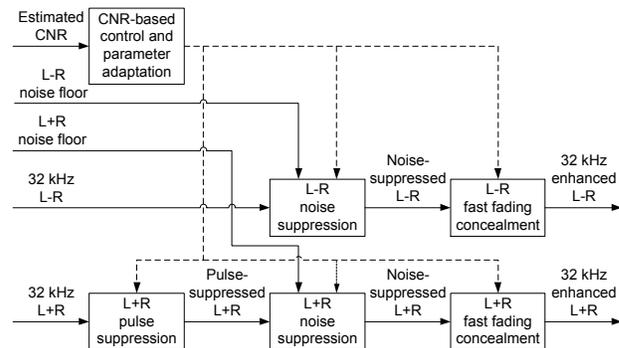
Figure 3 Back-end processing of FM enhancement systems
