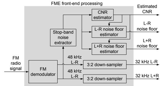
Figure 2 Front-end processing of the second FM enhancement system architecture
