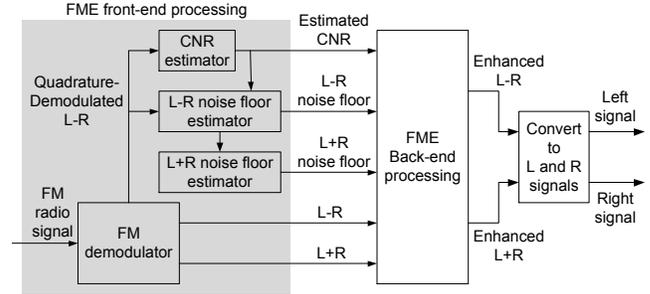
Figure 1 First FM enhancement system architecture
