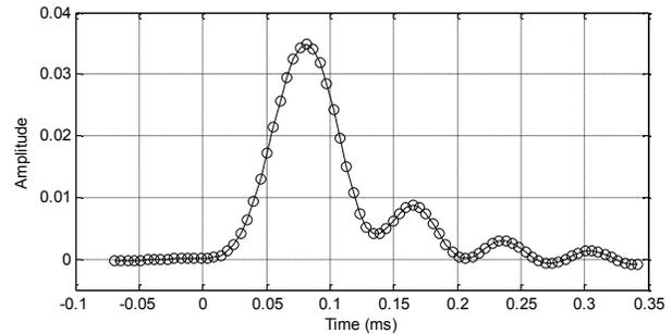
Figure 4 Prototype noise pulse at 192 kHz
