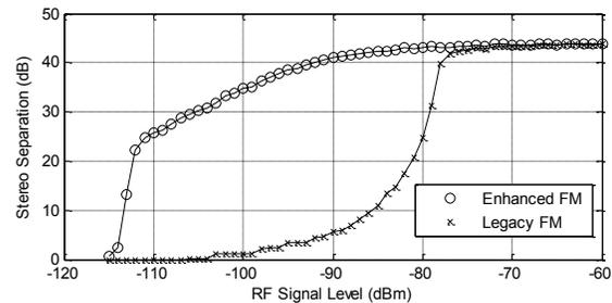
Figure 6 Stereo separation versus RF signal level
