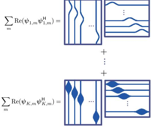
**Fig. 3.** Graphical illustration of  $\boldsymbol{\Psi}$ .  $\sum_m \psi_{k,m} \psi_{k,m}^H$  can be set at a circulant matrix in both cases of STFT and wavelet transform.
