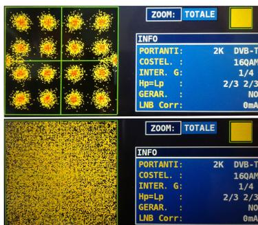
Fig. 8. Constellations received in intelligible zone (above) and interdicted zone (below).
