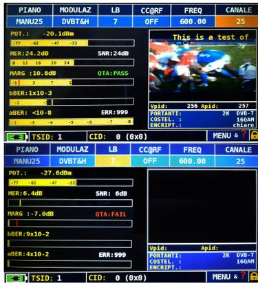
Fig. 7. Measured signal parameters as received in intelligible zone (above) and interdicted zone (below).
