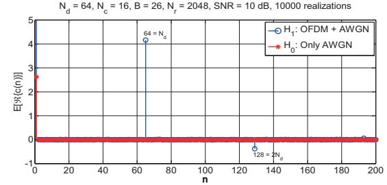
Fig. 2. A zoom of mean of real part of cepstrum of signals under  $H_0$  and  $H_1$  averaged over 10000 realizations and simulation parameters of  $N_d = 64, N_c = 16, B = 26, N_r = 2048, \text{SNR} = 10 \text{ dB}$ , 10000 realizations.  $\text{E}[Re[c(n)]]$
