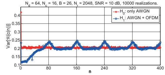
Fig. 3. Variances of cepstral coefficients under both hypotheses  $H_0$  and  $H_1$  averaged over 10000 realizations and simulation parameters of  $N_d = 64, N_c = 16, B = 26, N_r = 2048, \text{SNR} = 10 \text{ dB}$ . While variance plot of AWGN cepstrum is flat, presence of OFDM causes cepstrum to have pyramidal shapes peaking at the integer multiples of  $N_s$ .
