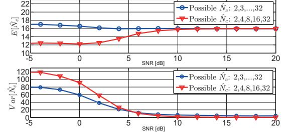
Fig. 7. Mean and variance of the  $\hat{N}_c$  value. Mean converges to the correct value 16 and variance reduces as the SNR increases. When the set of possible  $N_c$  values is finite containing a set of known possible values, the variance of  $N_c$  converges to zero.
