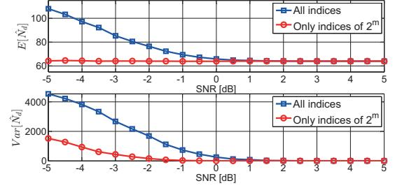
Fig. 6. Mean and variance of the estimate  $\hat{N}_d$ . The mean converges to the correct value 64 and variance converges to zero as the SNR increases.
