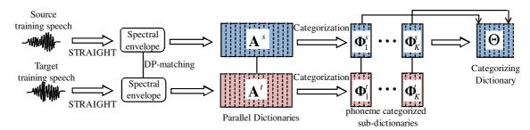
Fig. 3. Construction of categorizing dictionary that consists of representative vectors from each sub-dictionary.
