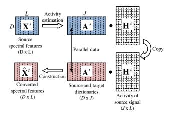
Fig. 1. Basic approach of NMF-based voice conversion
