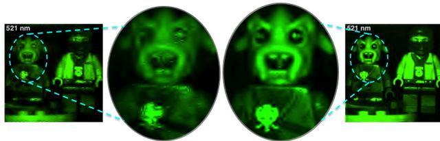
**Fig. 6.** Zoomed version of the reconstruction for the 5th spectral band using (Left) CASSI system, and (Right) colored patterned detector with 6 BP filters.
