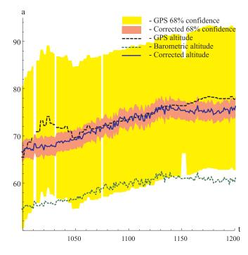
Fig. 4. Confidence bounds or GPS, barometric, and fused altitude measurements.
