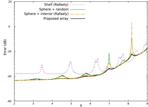
**Fig. 1.** Interpolation error for a plane wave inside the spherical arrays, for 50 trials at each wave number  $k \in [2, 9]$ . All the arrays have 130 microphones; the SNR = 40 dB.
