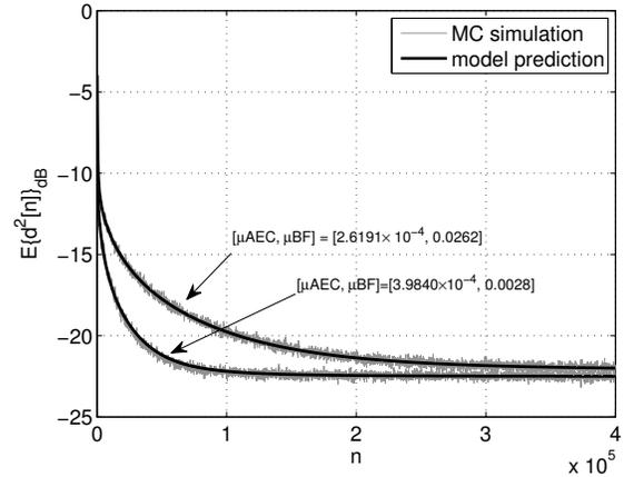
**Fig. 3.** Monte-Carlo simulation results for 20 runs with AR1(-0.9) input ( $M = 2$ ,  $N_h = 500$ ,  $N_{\text{BF}} = 16$ ,  $N_{\text{AEC}} = N_h + N_{\text{BF}} - 1$ ).
