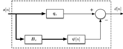
Fig. 2. BF-AEC system in the GSC configuration.
