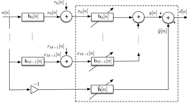
Fig. 1. BF-AEC system in the direct form structure [13].
