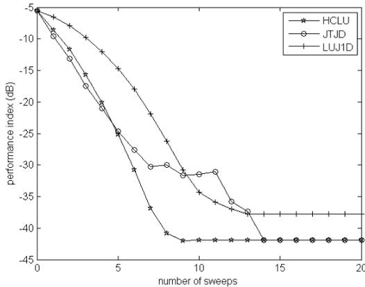
**Fig. 3.** Performances of the HCLU algorithm compared to the JTJD and LUJ1D algorithms when  $t = 10^{-2}$ .
