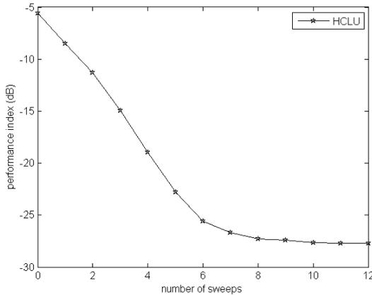
**Fig. 2.** Algorithms performances for 25 matrices of size  $15 \times 15$  with  $\mathbf{B}$  initialized as the identity matrix and with  $t = 10^{-2}$ .
