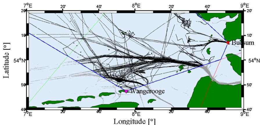
Fig. 2. AIS ship routes recorded on August the 4<sup>th</sup>, 2013.
