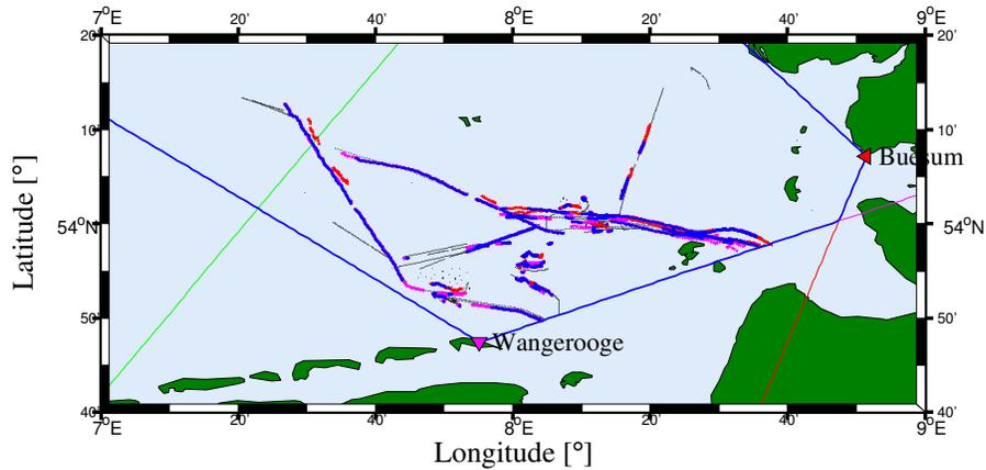
**Fig. 3.** True HFSW radar tracks and AIS routes on August 4, 2013 in the interval 00 : 00 – 02 : 00 UTC.
