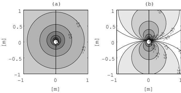
**Fig. 4.** Simulation results of the spatial responses of (a) omnidirectional and (b) dipole microphones.
