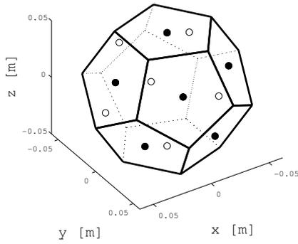
**Fig. 3.** Twelve-element spherical array
