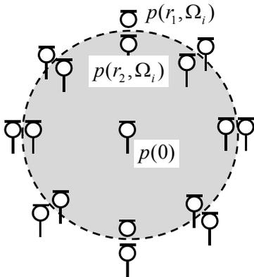
**Fig. 2.** Illustration of microphone positions and boundary surface in a conventional close-talking spherical array based on Kirchhoff integral equation.
