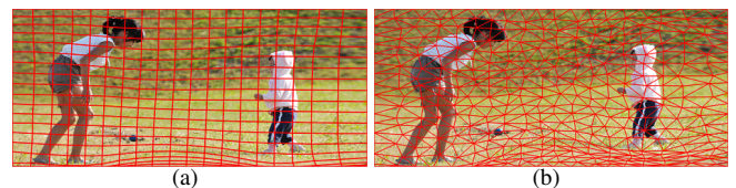
Fig. 5. Retargeting images with quadrilateral mesh (a) and triangle mesh (b).
