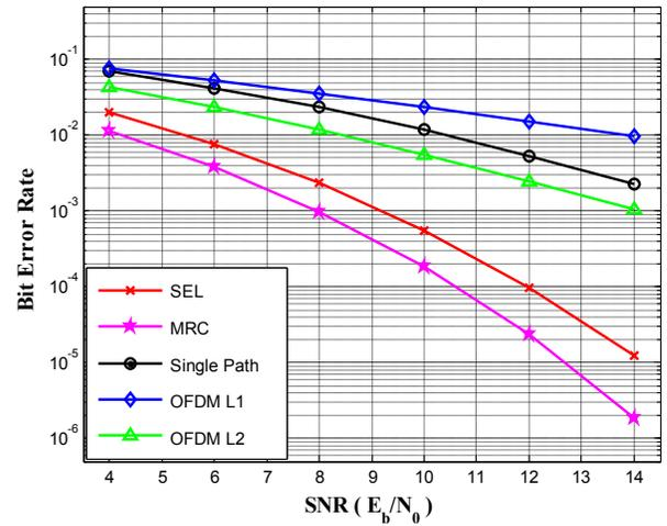
Fig. 6. BER over ITU-B Channel with 50 MHz Symbol Rate
