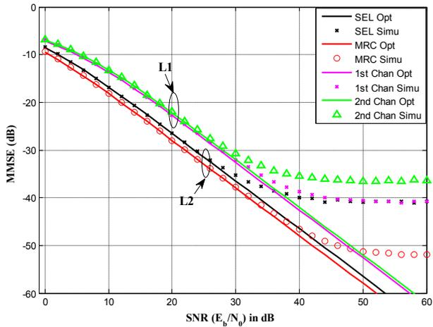
Fig. 5. MMSE after Linear Equalization for 1<sup>st</sup> Chan, 2<sup>nd</sup> Chan and Combined Channels
