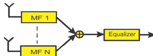
Fig. 1 Optimum Combiner / Linear Equalizer Structure
