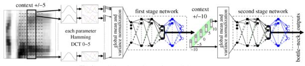
Fig. 1. Stacked Bottle-Neck Neural Network feature extraction.
