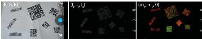
Fig. 4. Intermediate results rendered on the screen: original image; x-derivatives; edges (red) and corners (green)
