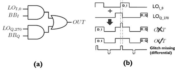
**Fig. 2.** (a) Functional logic and (b) signal waveforms of mixing cell
