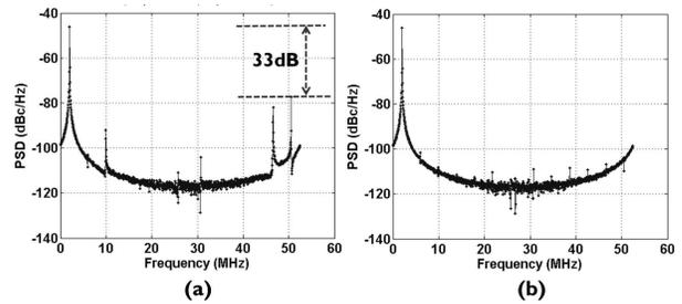
Fig. 7. PSD results before (a) and after (b) mismatch pre-distortion in the real-circuit simulation.
