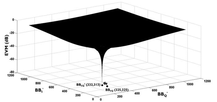
Fig. 4. EVM of the output corresponding to all the possible  $BB'_{I/Q}$ s for one given input  $BB_{I/Q}$
