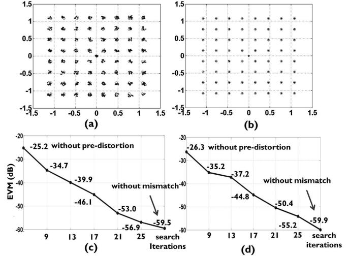
Fig. 6. 64-QAM constellation distorted by duty cycle mismatch (a) and after pre-distortion with 25 search iterations (b); EVM performance for 64-QAM (c) and 256-QAM (d).
