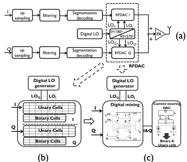
Fig. 1. Architecture of digital transmitter
