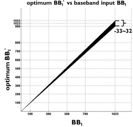
Fig. 3. Optimum  $BB'_I$  vs baseband input  $BB_I$
