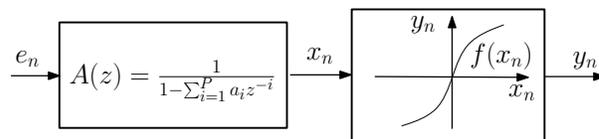
Fig. 1. Audio signal corrupted by memoryless nonlinearity.
