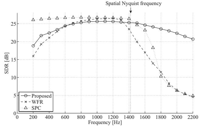
Fig. 5. Relation between SDR and frequency of source signal.
