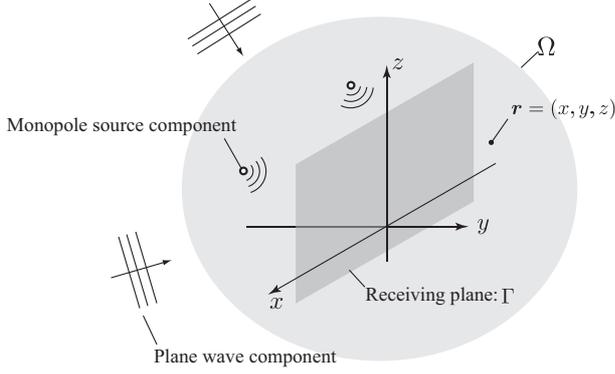
**Fig. 1.** Sound field in recording area is modeled by sum of monopole source and plane wave components. Sound pressure distribution is obtained by planar distribution of receivers.
