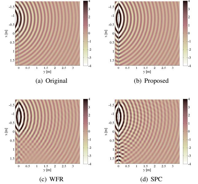
Fig. 4. Original and reproduced sound pressure distributions when source signal was 1.8 kHz. Spatial aliasing artifacts can be seen in WFR and SPC.
