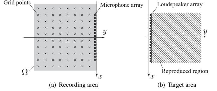
**Fig. 2.** Microphone and loudspeaker arrays are respectively set in recording and target areas. Region  $\Omega$  is discretized as set of grid points.
