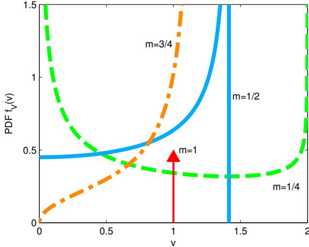
**Fig. 2:** The mixing distribution  $f_V(v)$  of Nakagami- $m$  fading envelope. When  $m = 1$  Nakagami- $m$  becomes Rayleigh, hence  $f_V(v)$  becomes a delta function, indicating that there is no mixing. The case  $m = 1/4$  does not belong to the Nakagami- $m$  family. Nevertheless it has well-defined mixing distribution and envelope.
