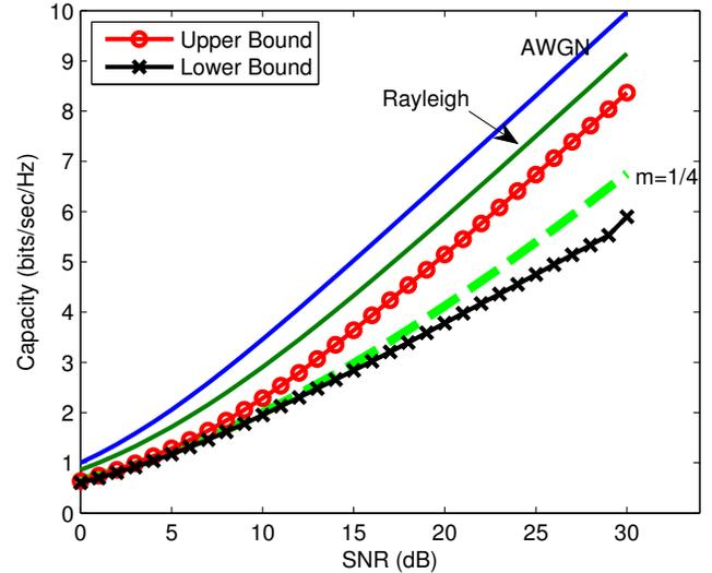
**Fig. 3:** The ergodic channel capacity of (7). With the non-Rayleigh constraint (24) we obtained tighter bounds that include the Nakagami- $m$  fading model with  $m = 1/4$  as a special case.
