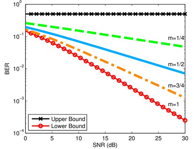
**Fig. 1:** The BER performance bounds for BPSK systems under uncertain SIRP fading statistic. The value  $m$  refers to the corresponding Nakagami- $m$  fading case. Note that for  $m = 1$  Nakagami- $m$  becomes Rayleigh, and it achieves the BER lower bound.
