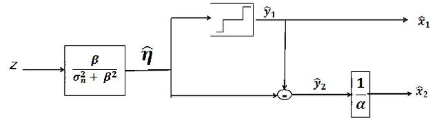
**Fig. 2.** Decoder of the SQLC scheme. Notice that the quantizer is the same as the one used in the encoder.
