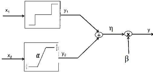
**Fig. 1.** Block diagram showing the SQLC encoder.  $x_1$  is passed to a uniform scalar quantizer of step  $\Delta$  and  $x_2$  is scaled and clipped to force it to lie within  $[-\frac{\Delta}{2}, \frac{\Delta}{2}]$ .
