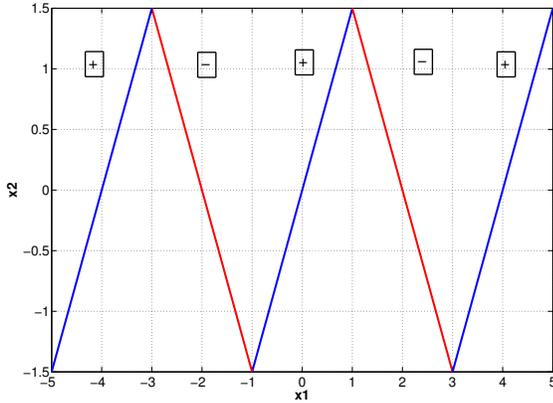
**Fig. 4.** Space filling curve for AS-SQLC. The two sources  $(x_1, x_2)$  are projected onto the curve and the resulting pair is transmitted as indicated in the text. Notice the *continuity* of the curve eliminating the threshold effect.
