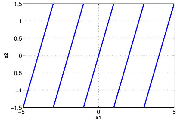
**Fig. 3.** Space filling curve utilized in the proposed system. Source symbols  $(x_1, x_2)$  are projected onto the curve to produce  $(y_1, y_2)$ .
