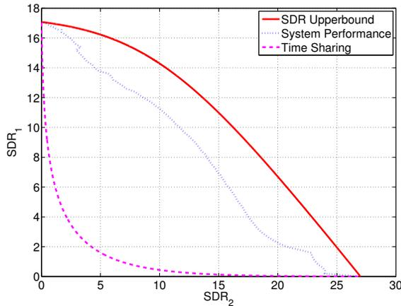
Fig. 7. System performance for  $P = 1$ ,  $N_2 = 0.002$  and  $N_1 = 10N_2$  for the optimal values of parameters  $\Delta$  and  $\alpha$ .
