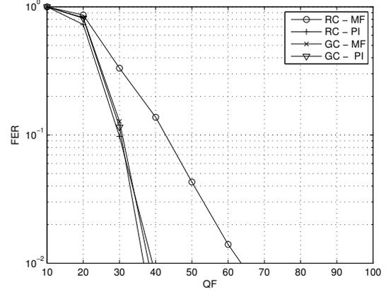
**Fig. 3.** FER performance of different encoding and decoding strategies in the presence of JPEG attack, considering nonblind decoding.
