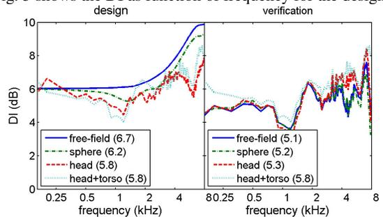
**Fig. 5.** Directivity index versus frequency for the bilateral microphone array with 4 microphones. Left: design. Right: verification.
