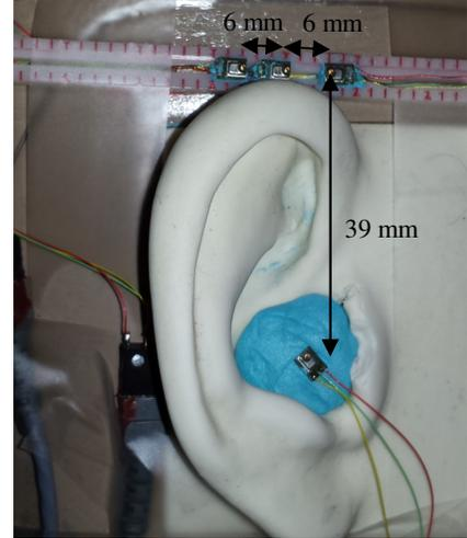
**Fig. 2.** The geometry of the microphone array on one-side of a manikin head.
