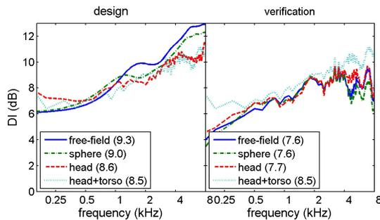
Fig. 7. DI versus frequency for bilateral microphone array with 4 microphones at each side. Left: design. Right: verification.
