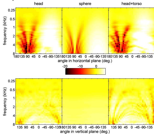
**Fig. 3.** Directional pattern as function of frequency and angle in the horizontal plane (top) / angle in the vertical plane (bottom) for head-only measurement (left) sphere simulation (center) and head+torso measurement (right).
