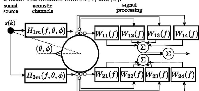
Fig. 1. Signal model for microphone array processing
