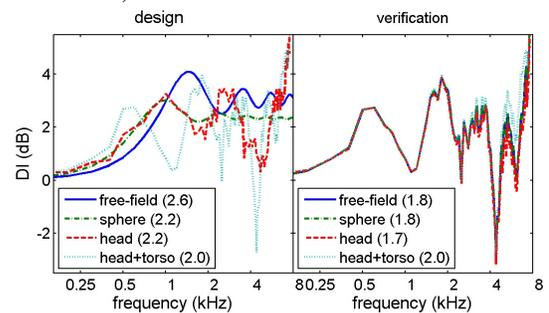
**Fig. 4.** Directivity index versus frequency for binaural microphone array with 1 microphone at each ear. Left: design. Right: verification.
