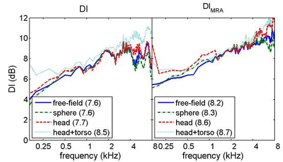
Fig. 8. DI (left) and  $DI_{MRA}$  as function of frequency.
