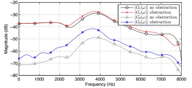
Fig. 5: Feedback paths' characteristics.
