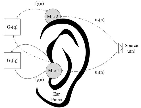
Fig. 3: Proposed microphone location.
