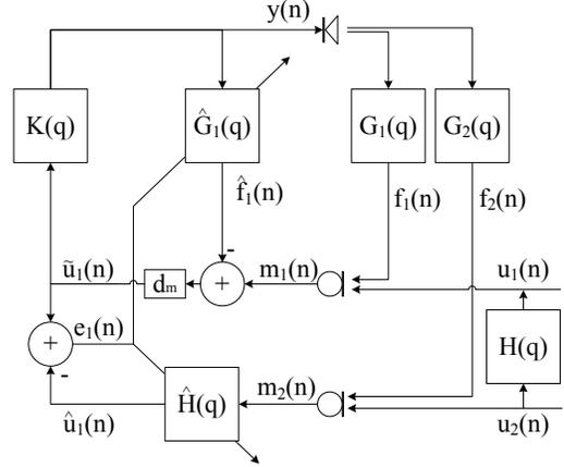
Fig. 2: TM-AFC set-up.
