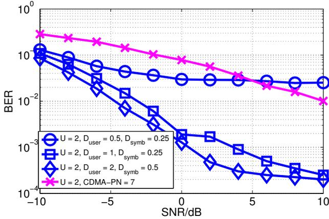
**Fig. 1.** Comparison between HFM-CDMA and new signaling scheme for varying  $D_{\text{symb}}$  and  $D_{\text{user}}$  for  $K=2$  users.
