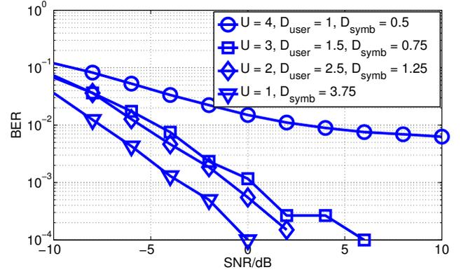
**Fig. 2.** Comparison between new signaling scheme for different number of users, where  $K=1, 2, 3, 4$  users with the best  $D_{\text{symb}}$  and  $D_{\text{user}}$  are chosen.
